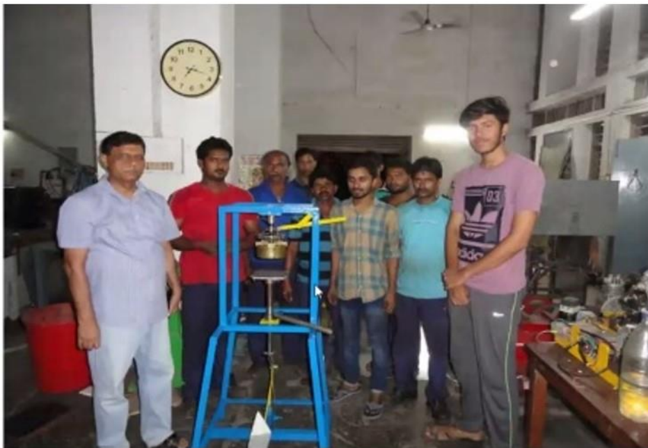
Pedal Operated Herbal Mosquito Repellent Coil Making Machine
